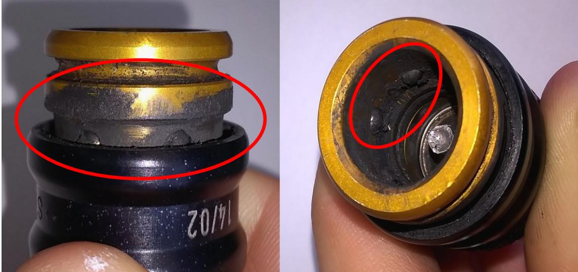
*Please ensure that the car-side quick release coupling is always clean & free of dirt, and if necessary the coupling should be lubricated with acid-free grease.*
