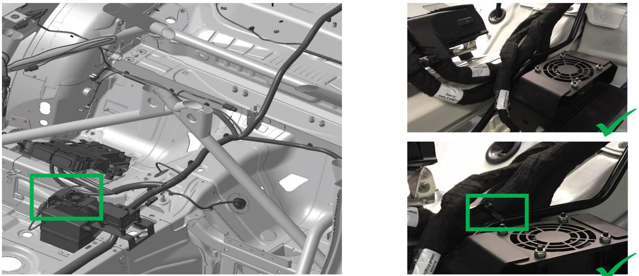
Porsche Motorsport informs users to be aware of the potential danger of chaffing on the car chassis loom section connecting the engine ECU. Chaffing can occur if the cable rests or is in contact with the top of the shift-compressor and its studs. Special attention should be made to avoid potential chaffing, e.g. sharp edges, when the body shell or wiring loom is exchanged.
