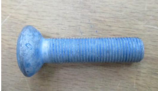
Attachment bolt with Porsche P/N: WHT.004.835 M12x1,25x4
