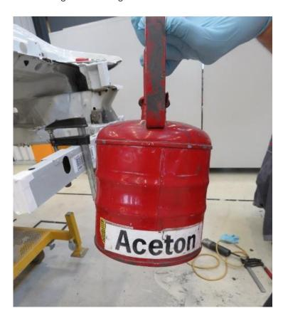
2. Clean the reinforcement plates and chassis using acetone.
