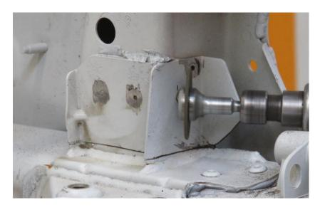
2. Grind off the rivet heads.
