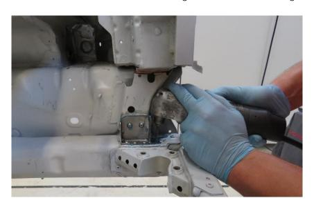
5. Bore out the lower rearward rivets holes using a 5 mm drill bit (use a drill bit with a length of 60 mm).
