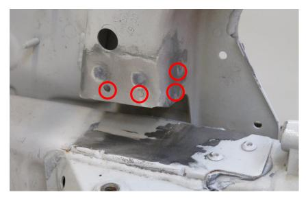
6. Use a punch / drift to knock out the rivet bodies (red circles).
