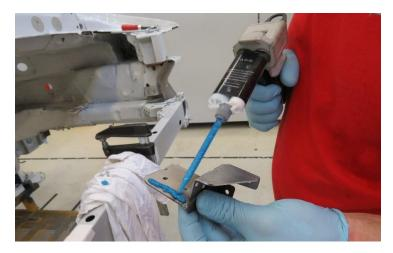
3. Apply the adhesive (Betamate 2096) to the reinforcement plates
