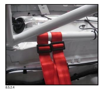
• Mount the shoulder straps in the same way as the shoulder straps of the driver on the harness bar of the safety cage.
