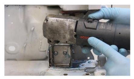
4. Bore out the lower front rivet holes using a 5 mm drill bit (standard length).
