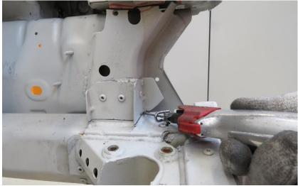
1. Cut off the old mounting using the body saw.
