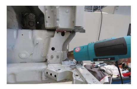
3. Use a hot air gun to heat the mounting and loosen the adhesive.
