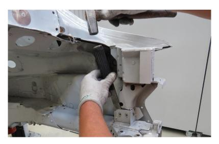
4. Remove the mounting using a hammer and chisel.
