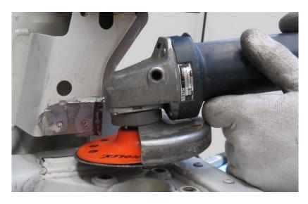
5. Remove any residual adhesive or steel residue.
