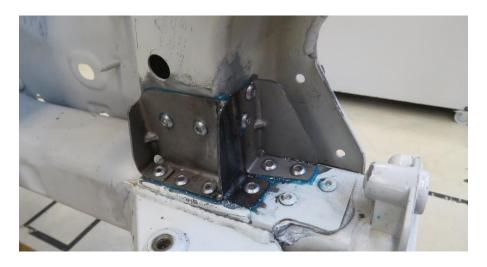
7. Remove any residual adhesive and clean the components.
