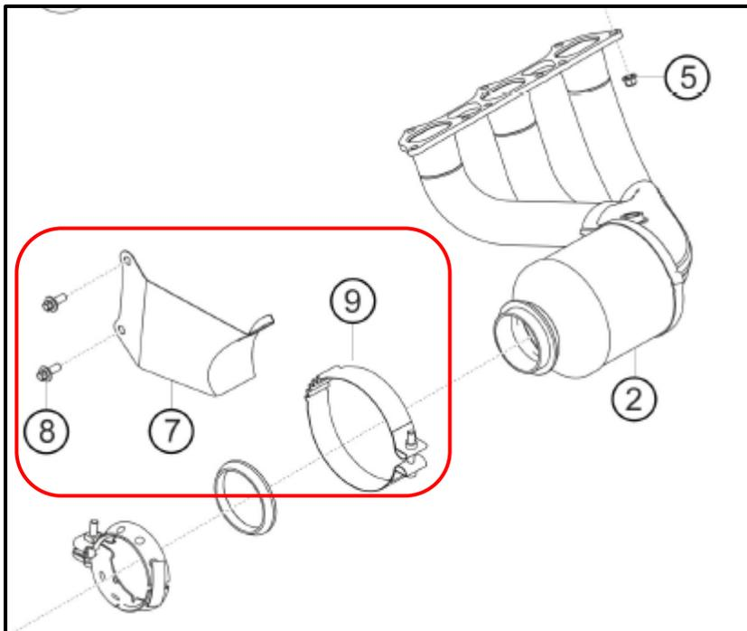
Porsche Motorsport informs that the bracket (7) for the exhaust manifold, the corresponding bolts (8) and the clamp (9) are now no longer required to fasten the exhaust manifold to the engine. These components must be removed when participating in Porsche One Make Cup events. Due to manufacturing reasons, new engines will continue to be supplied with the bracket. The mentioned parts should also be removed from new engines.
